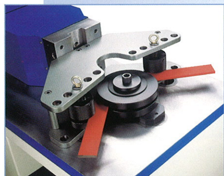
Flat plate edge bending tool for up to 50mm(w)x12mm(t)
